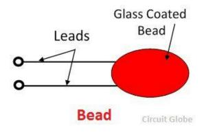
The bead form of the thermistor is smallest in shape, and it is enclosed inside the solid glass rod to form probes.
