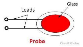
The disc shape is made by pressing material under high pressure with diameter range from 2.5 mm to 25mm.
