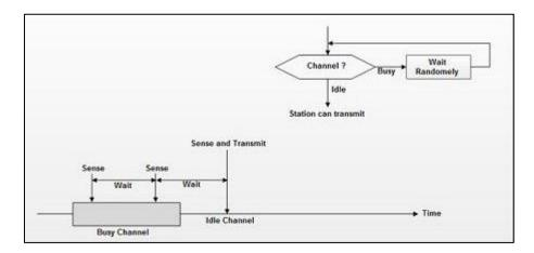
**P-Persistent:** The **p-persistent method** is used if the channel has time slots with a slot duration equal to or greater than the maximum propagation time. The *p*-persistent approach combines the advantages of the other two strategies. It reduces the chance of collision and improves efficiency. In this method, after the station finds the line idle it follows these steps:
