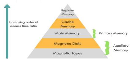
The total memory capacity of a computer can be visualized by hierarchy of components. The memory hierarchy system consists of all storage devices contained in a computer system from the slow Auxiliary Memory to fast Main Memory and to smaller Cache memory.
