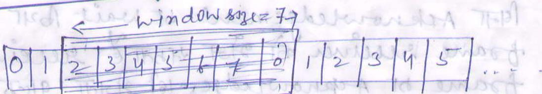
SL ↑ This wall move to right when a frame is sent      SR ↑ This wall move to right when an ACK is received.
