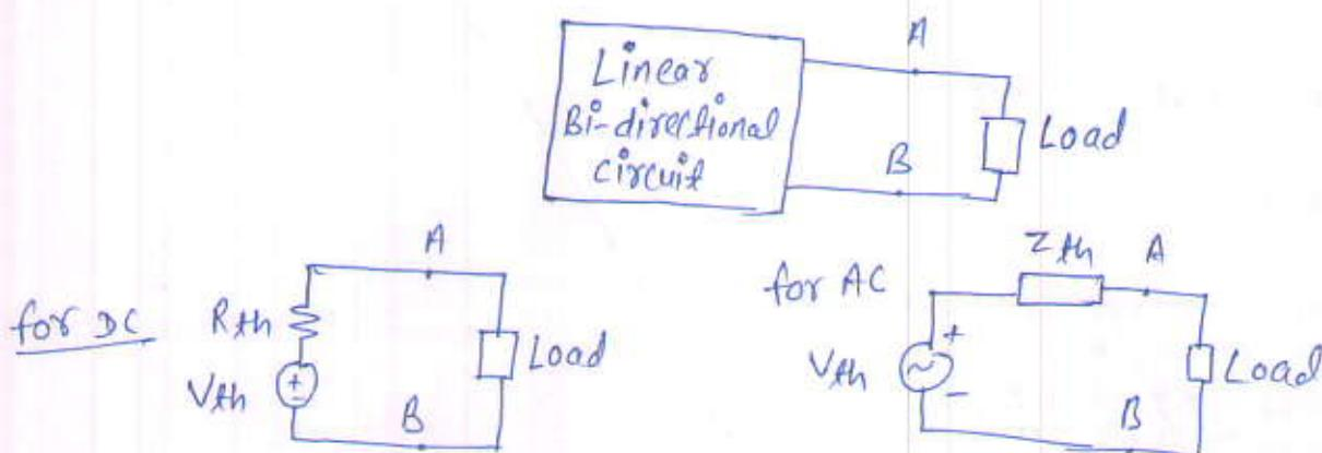
$V_{th}$ : - The Thevenin Voltage  $V_{th}$  is an ideal Voltage source equal to the open ckt Voltage at the Load terminals.
