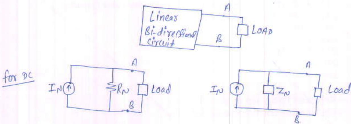
$I_N$ :- The Norton's Current  $I_N$  is an ideal current source equal to the short circuit current flowing through the Load terminal.
