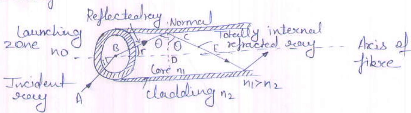
Interface at an angle  $\theta$ . Let  $\theta$  is greater than critical angle  $\theta_c$ . As long as the angle  $\theta$  is greater than  $\theta_c$ , the light stay within the fibre.
