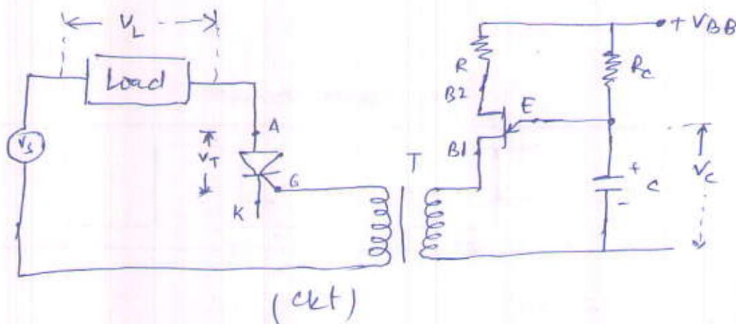
① The exact point of firing of SCR depends on appearance of gate pulse.
