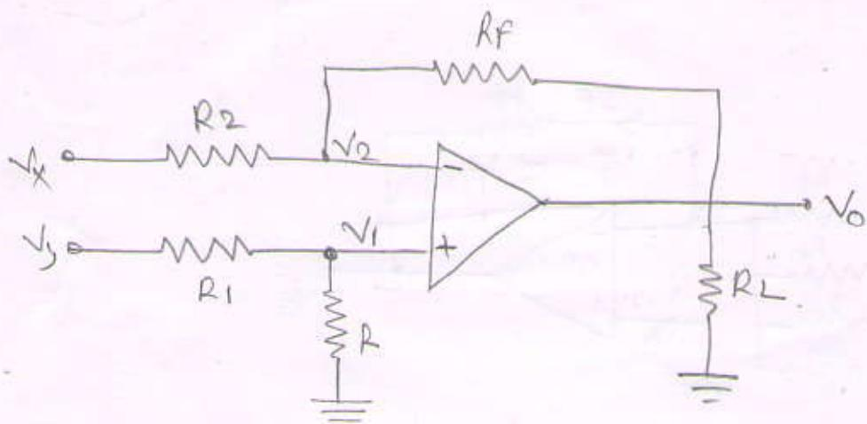
$$V_o = \frac{R_f}{R_1} [-V_y - V_x]$$
