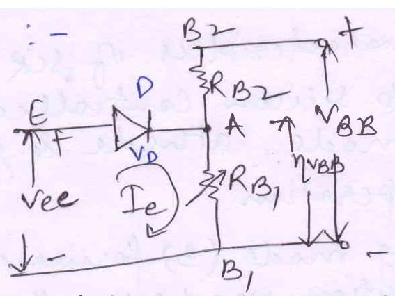
When volt  $V_{BB}$  is applied between base  $b_1$  &  $b_2$  than volt  $V_A = nV_{BB}$  & this volt acts as  $R_B$  on diode D. if  $V_{EE} < V_A$  there is no current flow in emitter due to Reverse biasing of diode. if  $V_{EE} > nV_{BB} + V_D$  than current flow through diode D.
