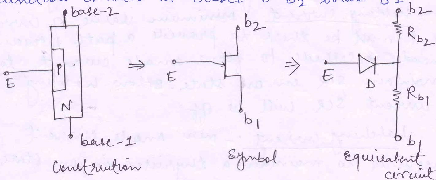
It is called unijunction transistor because there is single junction formed by embedding in of n-type Si base & p-type emitter.
