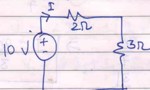
Calculating the current  $I$  in the circuit  $I = \frac{10}{5} = 2 \text{ Amp}$
