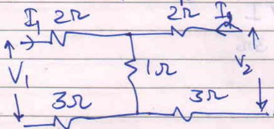
$$V_1 = 2I_1 + -1(I_1 + I_2) + 3I_1$$
