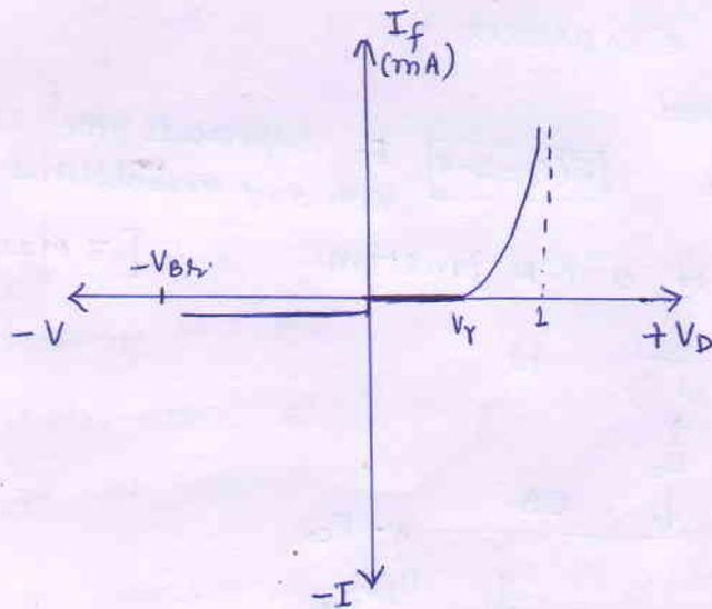
$V_r$  = cut-in voltage of Diode
