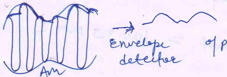
for  $\mu \leq 1$  envelope of AM signal will be  $m(t)$  so it can be demodulated by envelope detector. for  $\mu > 1$  message signal ~~can~~ not be recovered by this method
