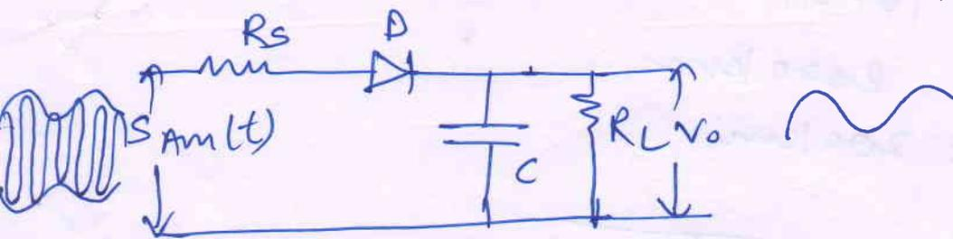
it is also called envelope detector. It is very simple & cheap. it extracts the positive envelope of modulated signal and gives off in this circuit capacitor is charged upto peak value of modulated wave and then discharge. but due to  $R_L C \ll$  radio frequency time constant capacitor ~~is~~ volt discharges very small and it again charged.
