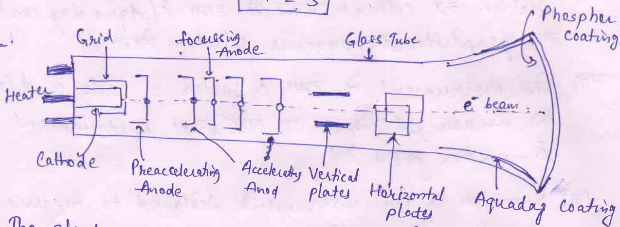
The electron gun contains an cathode which is heated indirectly by a filament; this results in the emission of  $e^-$  from the cathode surface.
