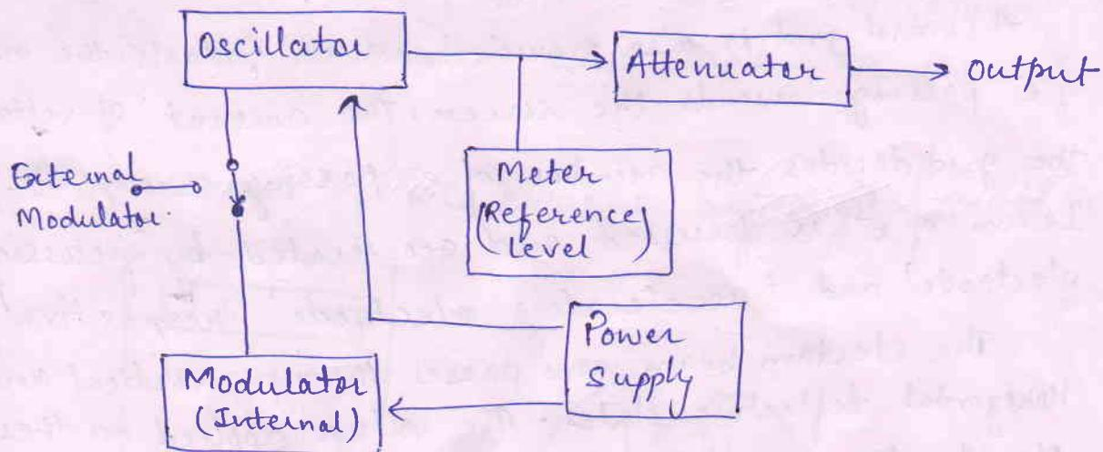
(v) Block Diagram of AF signal generator
