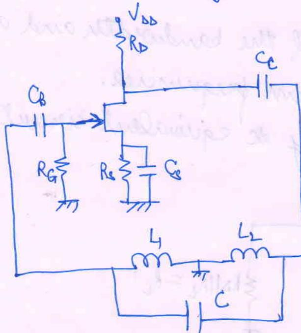
$C_B$  and  $C_F$  prevents the shorting and drain and gate with respect to ground.
