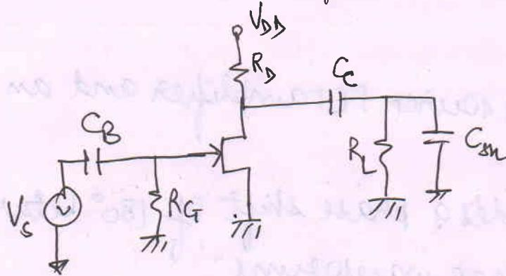
For the above circuit the source self bias configuration maintains the JFET in saturation region.
